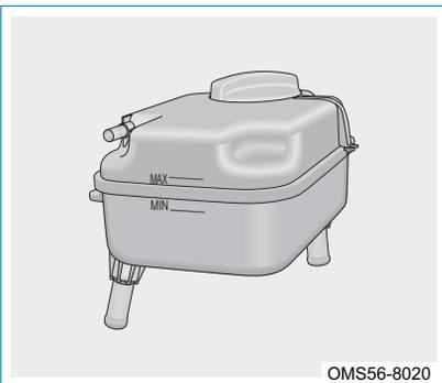
The vehicle must park on a level ground when checking coolant level. Check whether coolant level in reservoir is between MAX and MIN lines. If coolant in reservoir is boiling, the operation can be performed after coolant is cooled. If coolant level is lower than MIN line, add coolant to coolant reservoir according to specified procedure.
