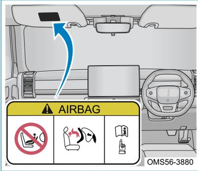
Labels are attached to front passenger side sun visor, indicating that it is forbidden to install a rearward-facing child restraint system on the front passenger seat. Be sure to observe the following precautions:
