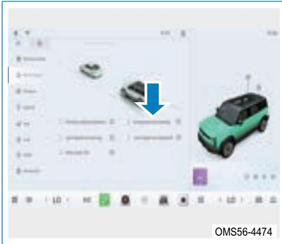
Click "Vehicle" in the audio system to select "Smart Driving", and click "-Emergency Lane Keeping" switch to turn it on or off.
