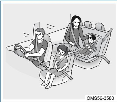
We strongly recommend the driver and passengers wear their seat belts correctly at all times. Failure to do so could increase possibility and severity of injury in case of an accident. Check the seat belt regularly. If any seat belt function failure is found, please contact authorized service station immediately to inspect, repair or replace the belt.
