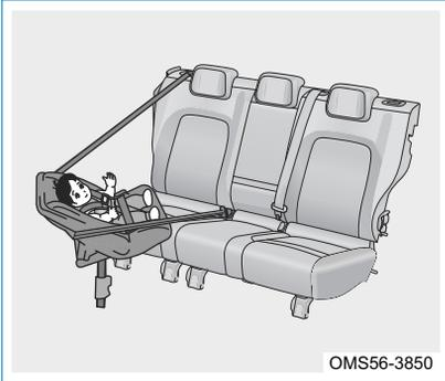
When installing the rearward-facing infant seat, ensure that it is installed towards the rear of the vehicle. If a baby faces the front of the vehicle in an accident, it is likely to injure their delicate central spine and spinal cord. When the baby faces the rear of the vehicle, their head, neck and torso are protected by the protective seat. The rearward-facing infant seat is the most suitable for infants and is very easy to carry. It is recommended for level 0 and 0+.
