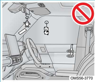
Do not attach anything to areas such as the door, windshield glass, side door glass, A pillar, B pillar, C pillar, roof side rail and assist grip.
