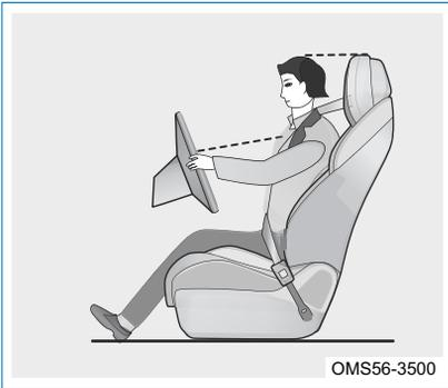
The shoulder belt should be over the center of the shoulder and close to the chest, kept away from the neck, the lap belt should lie over the hips but not stomach.
