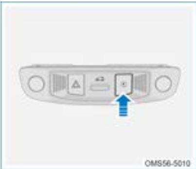
Long press the emergency power-off switch for 3 seconds or press the emergency power-off switch continuously for 3 times within 3 seconds, the vehicle power is off.
