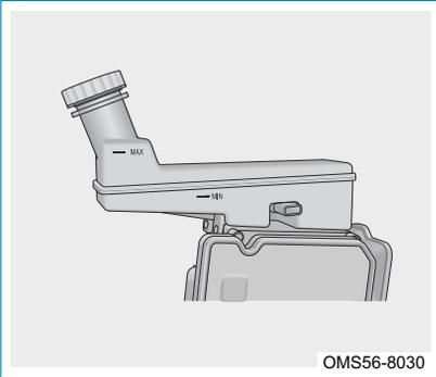
Brake fluid level should be between the "MIN" and "MAX" marks. If the level is at or below the "MIN" mark, add brake fluid and contact authorized service station for inspection and repair immediately.
