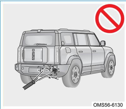
High pressure water flow such as water guns or excessive external forces may cause damage to the sensor. Do not pinch or impact the sensor, or it may cause abnormal operation.
