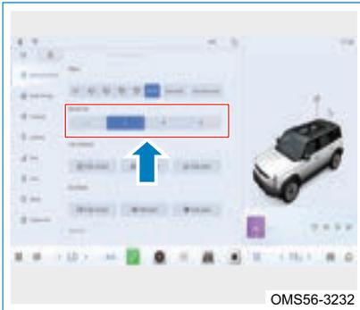
If you need to control the wiper frequency more accurately, you can set the wiper sensitivity in this screen of audio system in auto mode.
