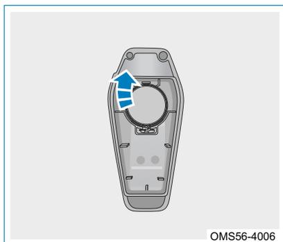
2. Remove battery from circuit board and install a new one with positive (+) facing up.
