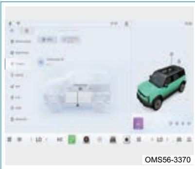
High power reverse discharge function: This function has a lower limit setting for remaining power usage, which is 20% by default. When setting it by yourself, the maximum remaining power limit can only be adjusted to -10% lower than the current remaining power. If the setting is higher than the current remaining power, it will be prompted that the power is low, the reverse discharge function cannot be turned on, and the remaining power limit needs to be reset.
