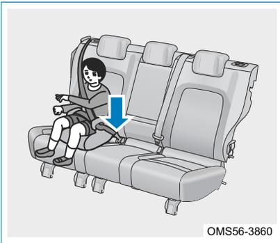
After installing the forward-facing child restraint system, the child faces the normal driving direction of the vehicle. Recommended for level I: 9 ~ 18 kg.
