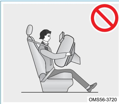
Always keep airbag inflation path clear. It is forbidden to place anything (mobile phone, etc.) between the occupant and the airbag. It is forbidden to fix or place any object on or near the airbag cover. If there is an object between occupant and airbag, the airbag may not deploy according to design path, or the airbag may push object to occupant's body, causing serious injury or even death.
