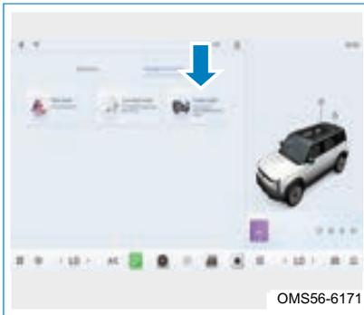
Before towing, you need to turn on towing mode through head unit display.
